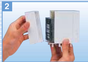
Remove the back cover of the main unit.
