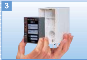
Remove the old sensor unit and reload the new sensor unit.
