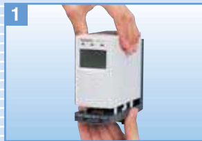
Remove the main unit from the base unit.
