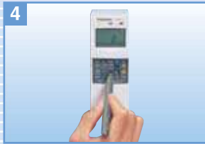
Mount the main unit on the base unit and press the test switch to confirm operation.
