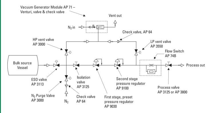
Note: This schematic is intended as an example of AP Tech component usage only. It does not include pressure measurement, filtration, etc. which must be included in a system.
