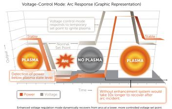
Voltage-Controlled Arc Response  $\rightarrow$  Faster Arc Recovery  $\rightarrow$  Increased Yield
